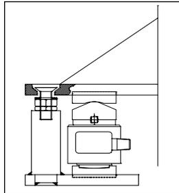
If the mount does not offer uplift protection, one may be established externally as per the drawing opposite. The uplift protection should be adjusted with a clearance of at least 1mm and requires regular inspection of this clearance.
