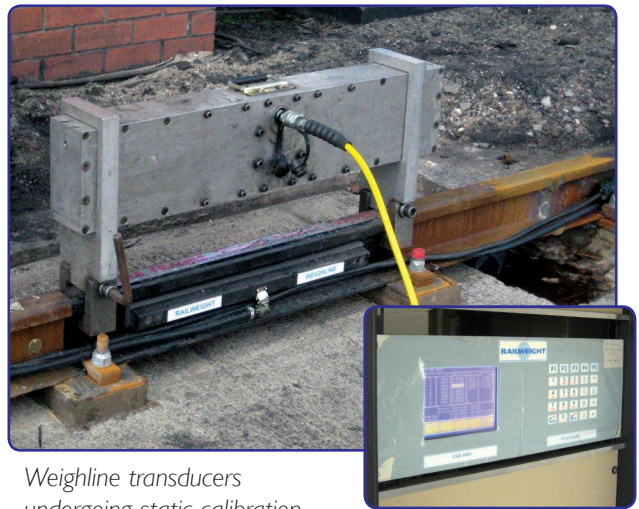
Weighline transducer rails being installed
