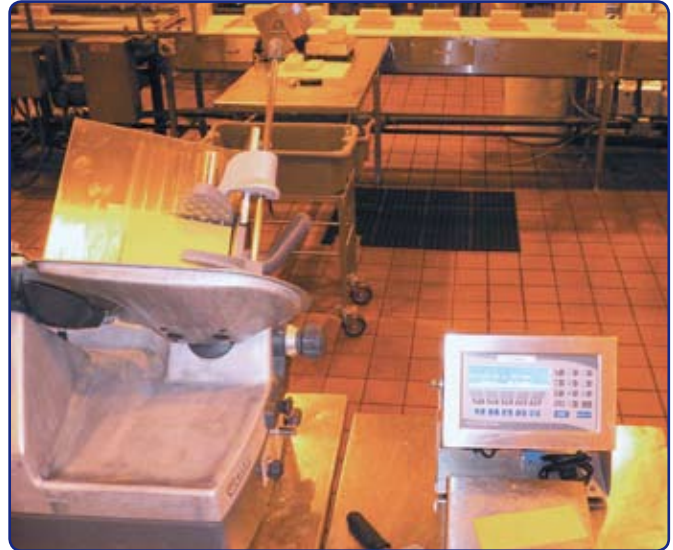
TCCA uses a high-speed checkweigher on the production line that verifies the weight of each cheese loaf. If a loaf is over or underweight, the Avery Weigh-Tronix E1310 checkweigher determines how much cheese should be removed or added.
